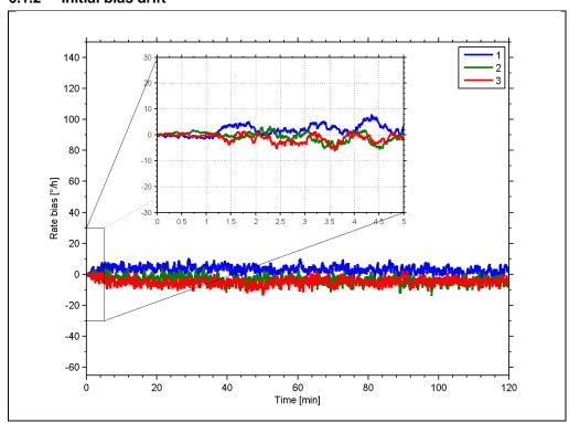
Figure 6-4: Typical normalized initial bias drift
