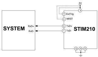
Figure 8-1: Transmit-Only Electrical Connection Diagram
