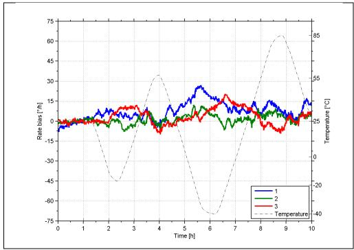
Figure 6-5: Typical Bias drift over temperature
