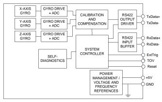
Figure 1-1: STIM210 FUNCTION BLOCK DIAGRAM
