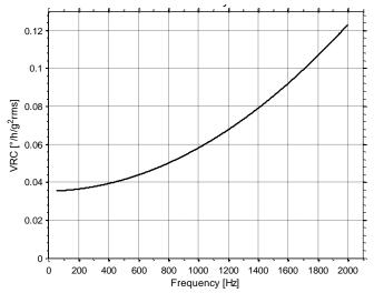
Figure 6-1: Nominal VRC at 5g rms for gyros
