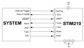
Figure 8-2: Full Function Electrical Connection Diagram
