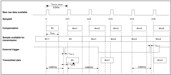
Figure 8-3: Timing of external trigger
