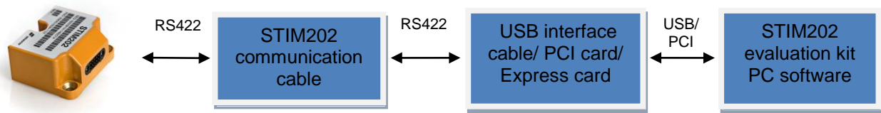
Figure 3: STIM202 evaluation kit connections/setup schematics
